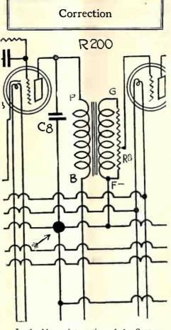
In the blue print section of the September issue, page 19, the circuit diagram of the Radio Age 6-Tube A C Receiver does not show the grid returns connecting to negative B lead. The correction is illustrated in the accompanying section of the original circuit lay-out.
