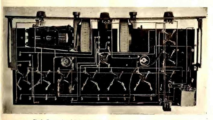
Fig. 3. Bottom view of the superheterodyne showing simplicity and neatness of wiring
