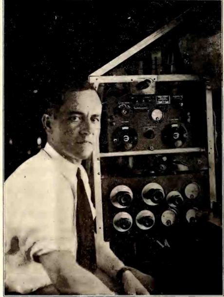
Ensign S. V. Edwards, U. S. N., seen at the radio set he will operate in the huge Sikorsky plane recently built for trans-Atlantic flights. The set is designed to be capable of sending and receiving messages from France or the United States as soon as it takes the air, having both a low and long wave length. The set weighs 125 pounds and was built by the Washington Navy Yard.—*Pholo copyright by Henry Miller*.
